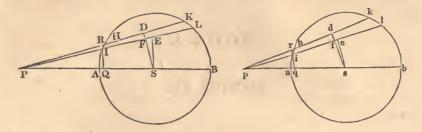
PIL very near each other, and SFD, SE perpendicular upon them, and from (p) draw phk, pil, so that hk, il may equal HK, IL respectively, and sfd, se, ir perpendiculars upon them may equal SFD, SE, IR respectively; then ultimately PE = PF = pe = pf, and DF = df. Draw IQ, iq perpendicular upon PS, ps.
